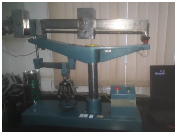
Plate 3-2. Instrument Used to Measure Modulus of Rupture
