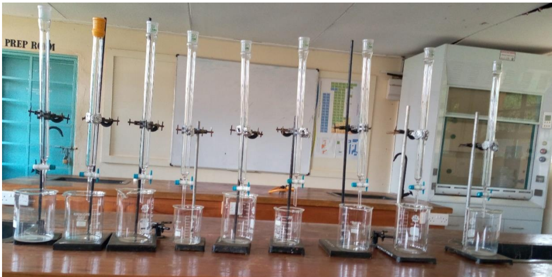
Figure 3.2: Illustration of the columns in which biochar was packed
