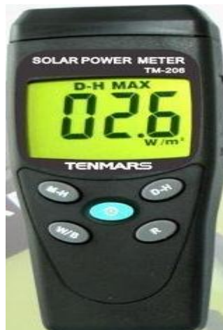
Figure 3. 2: Solar power intensity meter
