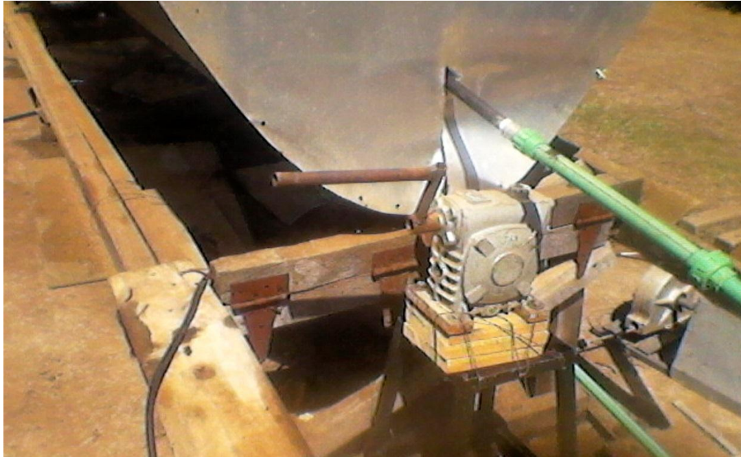
Plate 16: Solar gear tracker with lever in position during tracking
