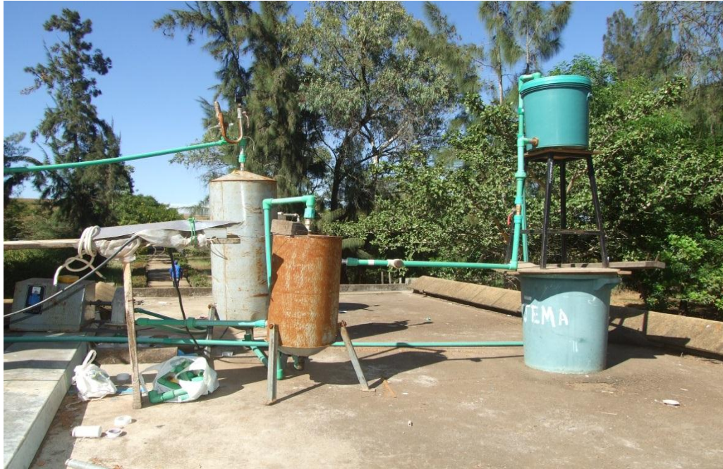
Plate 12: Solar thermal collection for vegetable oils
