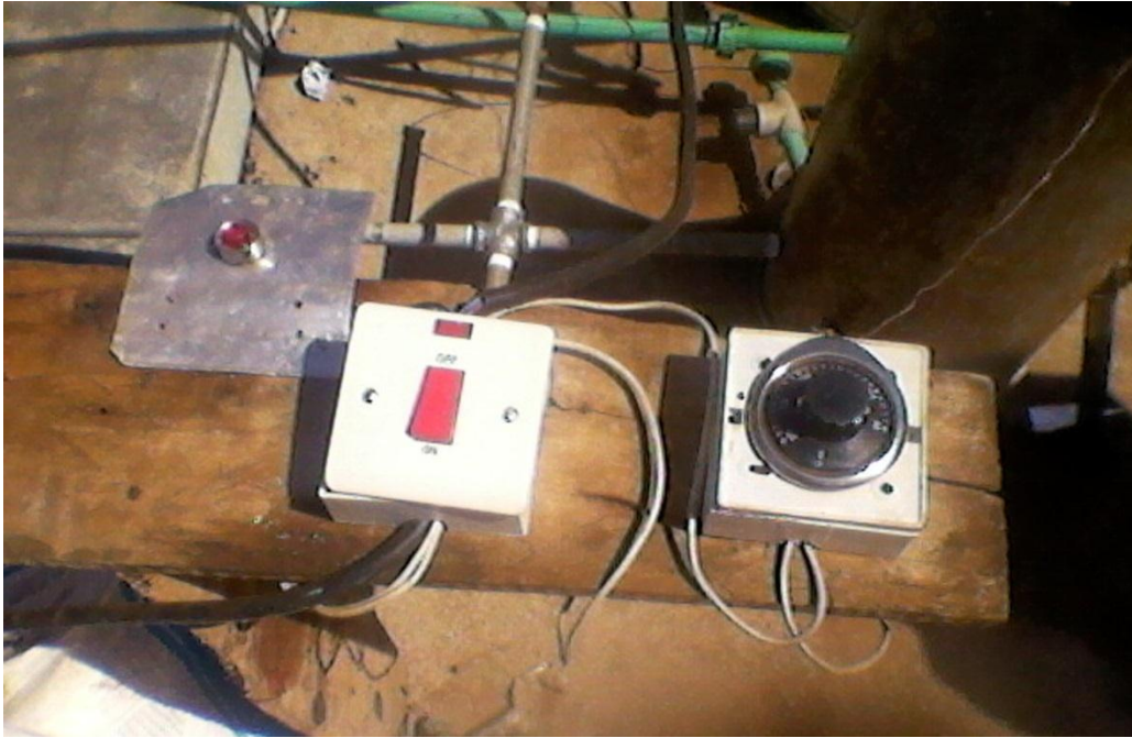
Plate 15: Power source and thermostat for testing loop
