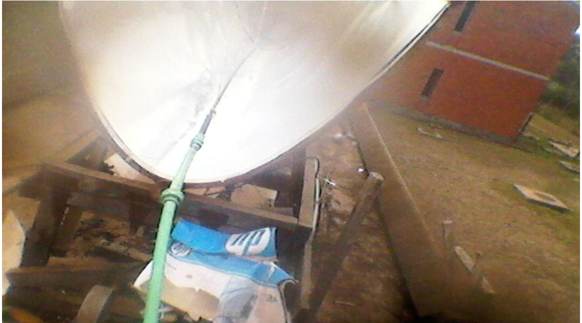
Plate 18: Receiver in position during oils solar thermal collection
