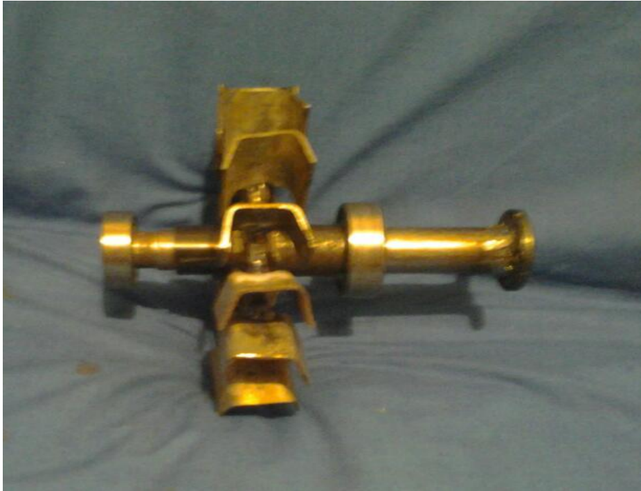
Plate 5: Turbine blades riveted to shaft
