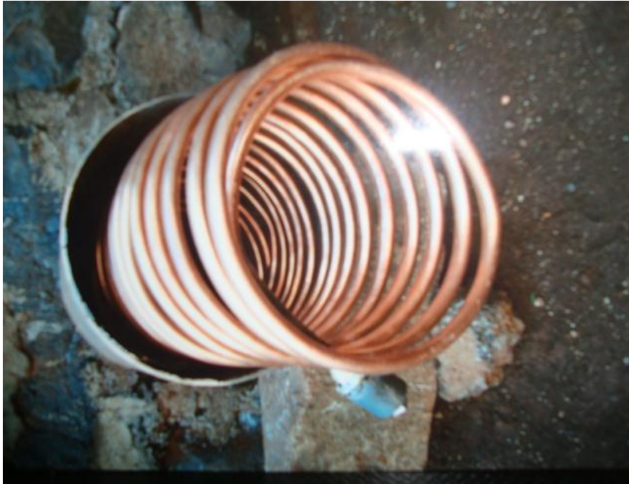
Plate 3: Heat exchanger with copper tube
