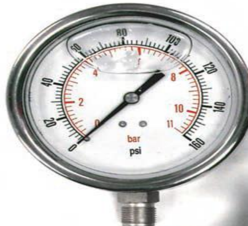
Figure 3. 1: Bourdon tube gauge
