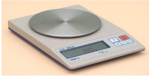
Figure 3. 5: The Electronic balance used in the study.
